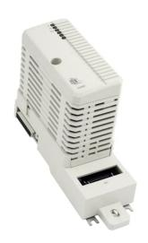
S100 I/O communication is realized in AC 800M by communication interface C1856, which is connected to the CEX-Bus through a base plate. The baseplate, TP856, houses a ribbon connector connecting to bus extender boards in S100 I/O racks and provides a simple DIN-rail mounting. Up to five S100 I/O racks can be connected to one C1856 where each I/O rack can hold up to 20 I/O boards.
