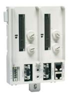
The TU847 is a module termination unit (MTU) for redundant configuration of the field communication interface CI840/CI840A. The MTU is a passive unit having connections for power supply, electrical ModuleBus, two CI840/CI840A and two rotary switches for station address (0 to 99) settings. A ModuleBus Optical Port TB842 can be connected to TU847 via TB806.
